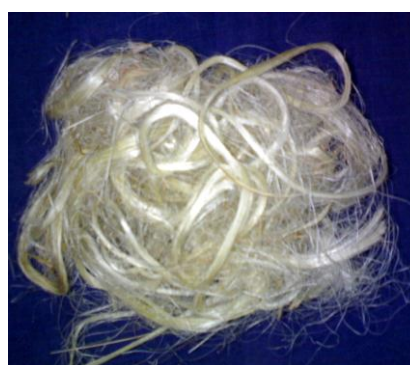
Fig. 2: Fiber Yield after Retting Process.
