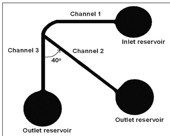
**Fig. 1:** Schematic Diagram of the Microchannel Bend is Shown (top view).
