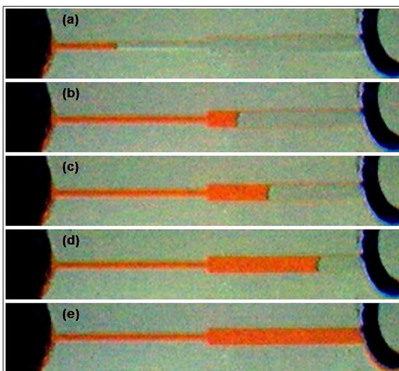
**Fig. 2:** A Representative-group of Snapshot Images is Showing the Surface-driven Capillary Flow of Dyed Water in the Sudden Expansion Microchannel with Expansion Ratio of 1:4.
