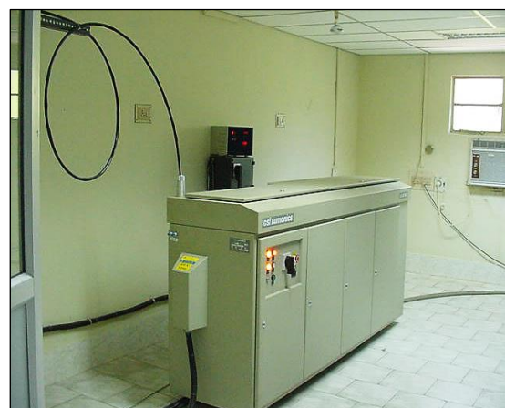
Fig. 1: Solid State Nd:YAG Laser Source at WRI Used for Experimental Work [25].
