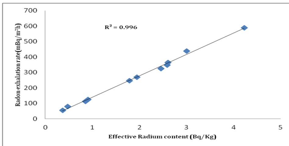
**Fig. 4:** Correlation Between Radon Exhalation Rate from Building Material Samples and the Effective Radium Content.
