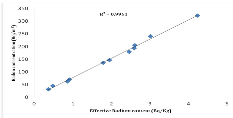
**Fig. 5:** Correlation Between Radon Concentration of Building Material Samples and the Effective Radium Content.
