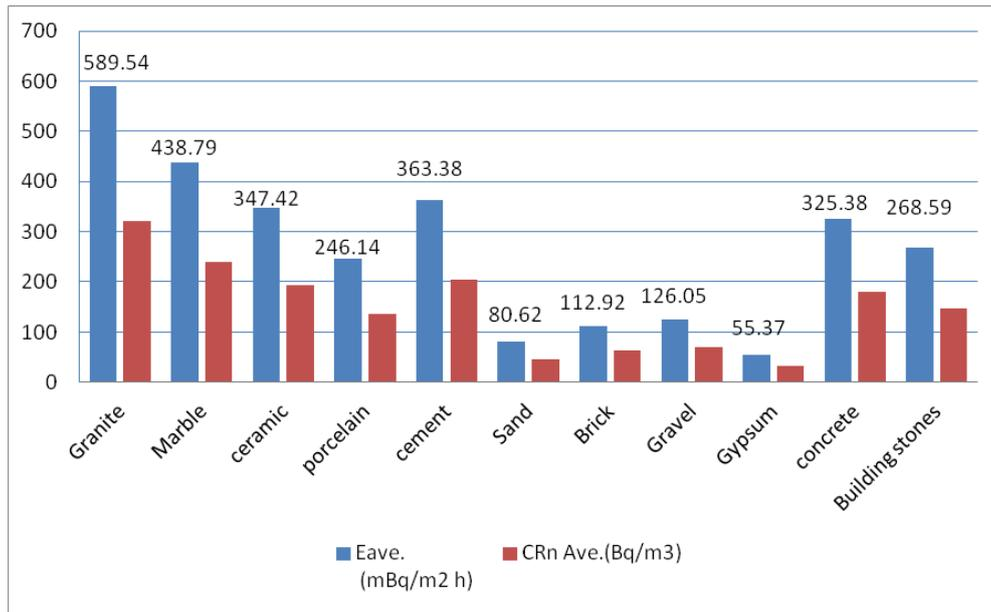
**Fig. 3:** Comparing Histogram for the Average Radon Concentrations ( $C_{m Ave.}$ ) and Exhalation Rates ( $E_{Ave.}$ ) from Building Materials.
