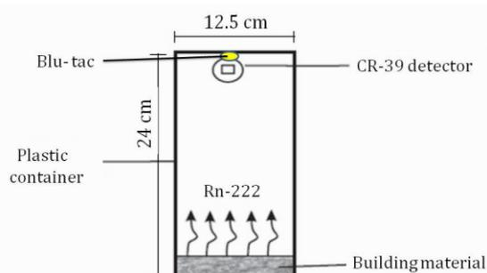
**Fig. 2:** Experimental Setup for the Measurement of Radon Exhalation Rate.
