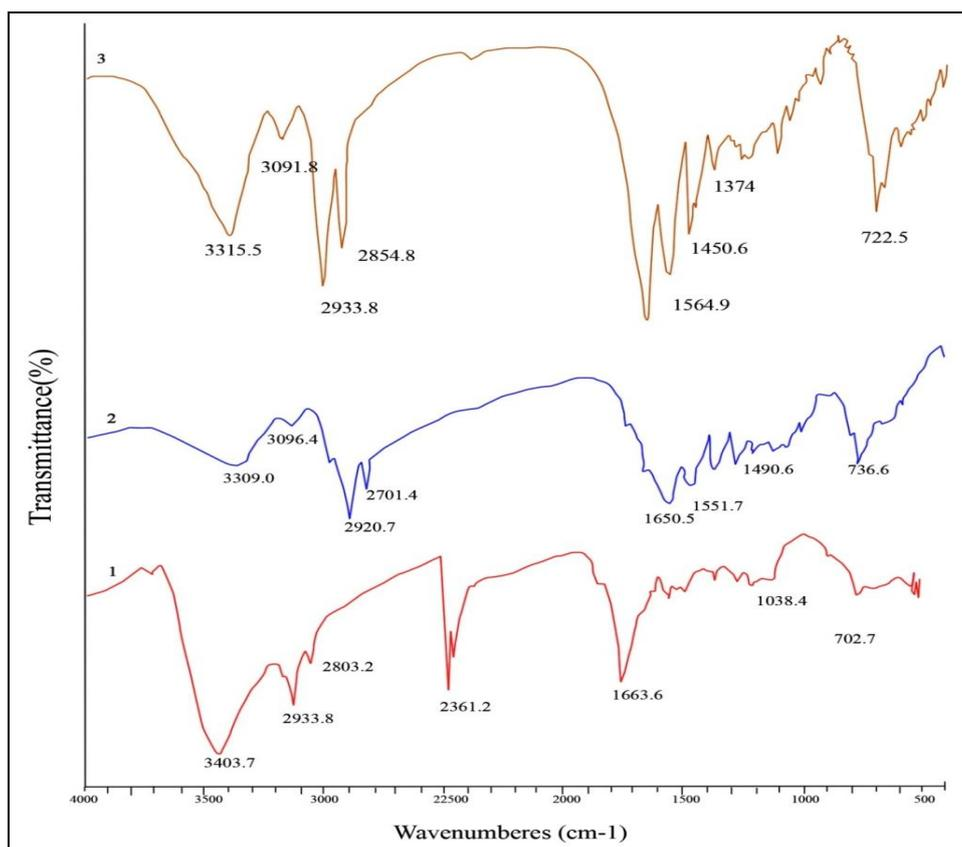
**Fig. 7:** FTIR Spectra of Irradiated PA6/PA12 Copolymer with Different Compositions: Curve 1 PA6; Curve 2 5/95; Curve 3 10/90.
