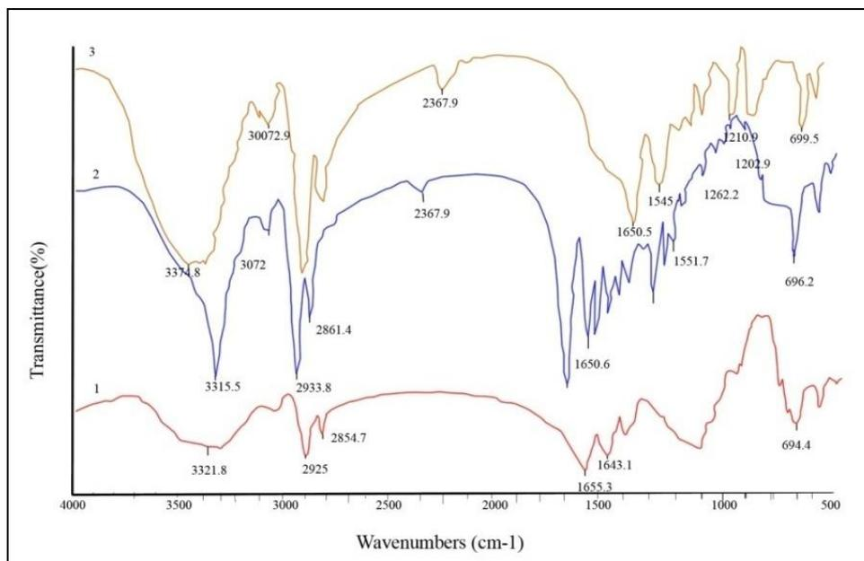
**Fig. 6:** FTIR Spectra of Irradiated PA6/PA12 Copolymer with Different Compositions: Curve 1 PA6, Curve 2 5/95, and Curve 3 10/90.
