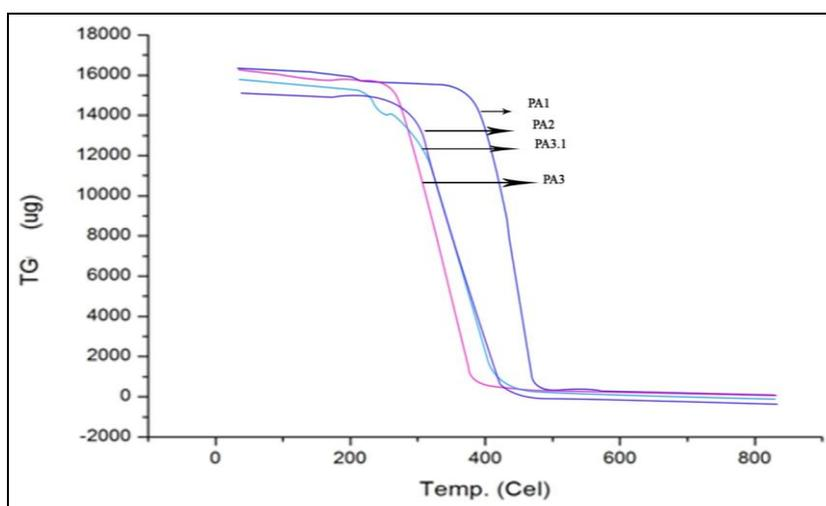
**Fig. 2:** TGA Thermogram of PA6/PA12 Copolymers.
