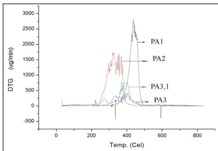
**Fig. 3:** Differential Thermo Gravimetric Analysis (DTG) of PA6 Copolymers.
