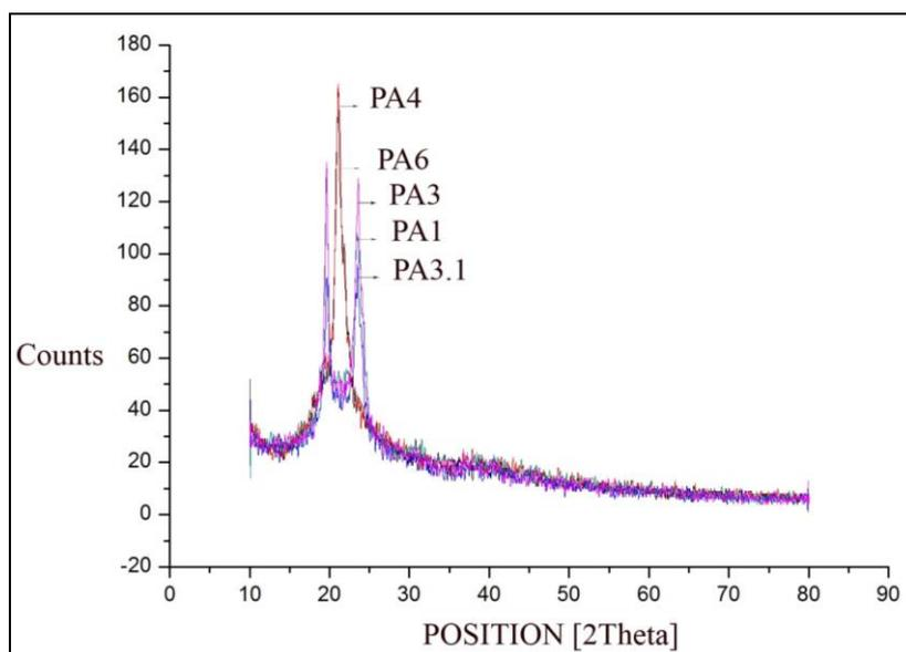
Fig. 4: X-Ray Diffractograms of PA6 Copolymers.
