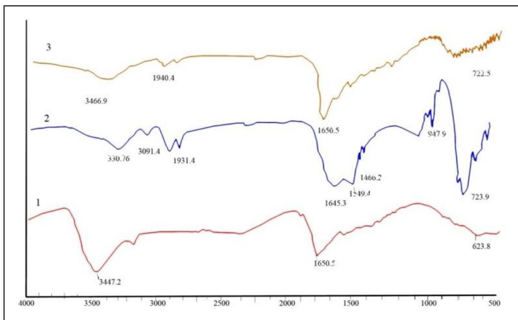
Fig. 5: FTIR Spectra of PA6/PA12 Copolymer with Different Compositions: Curve 1 5/95, Curve 2 10/90, and Curve 3 20/80.
