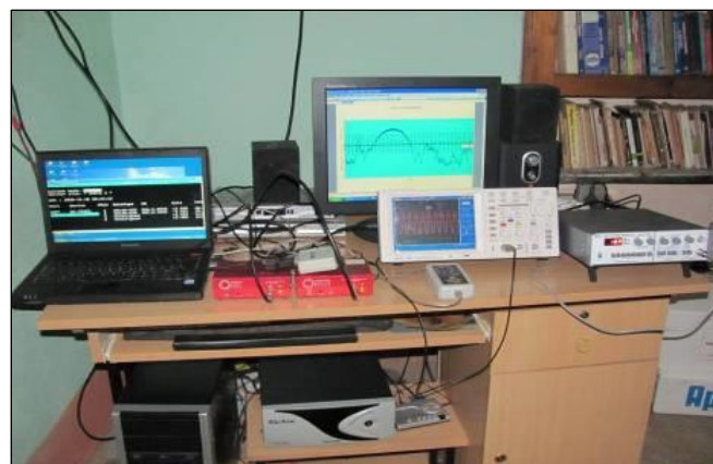
Fig. 2: Experimental Set up -Two Channel VLF Field Strength Monitoring System.
